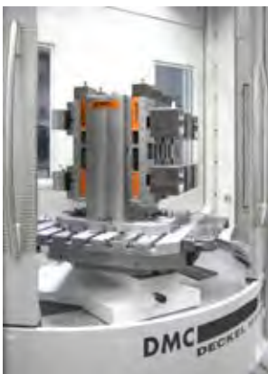
6-compartment design DUO 125 on double bracket
